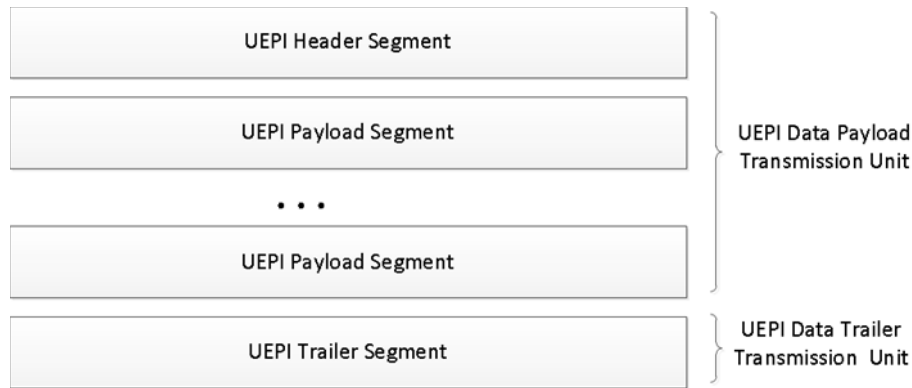
Figure 9 - UEPI Data Pseudowire Payload and Trailer Transmission Units for an OFDMA Channel
