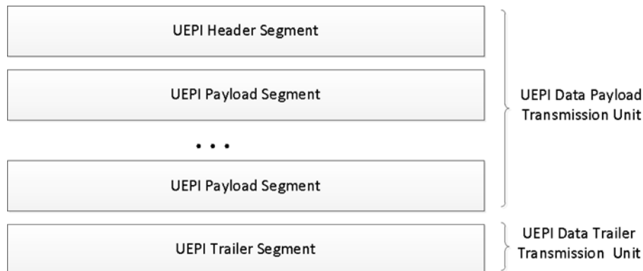
Figure 10 - UEPI Data Pseudowire Payload and Trailer Transmission Units for an OFDMA Channel
