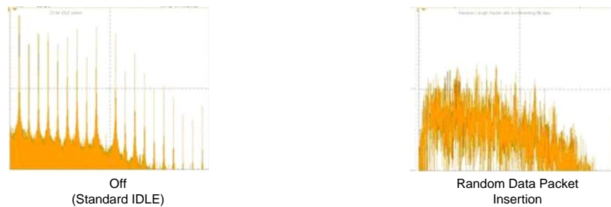
Figure 4 - Interference Spectra Without and With Raman Mitigation
