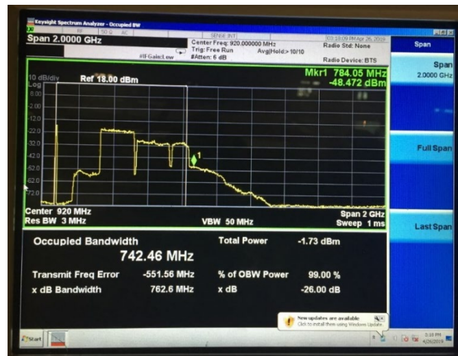
Figure 110 - Spectrum Analyzer Display of Downstream Signal with High Laser Distortion, OFDM RxMER = 23 dB
