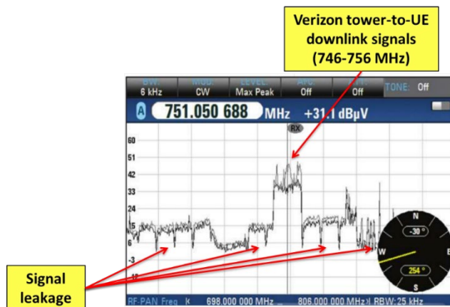
Figure 126 - Cable Network Signal Leakage in the 700 MHz LTE Spectrum, Overlapping LTE Band 13 (Verizon) Tower-to-UE Downlink Signals
