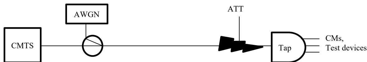
Figure 135 - Test Setup for Test Sets A and B
