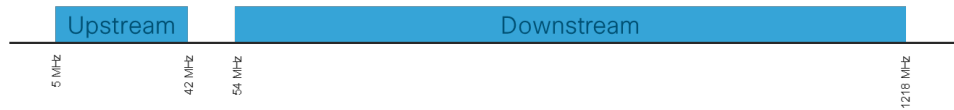
Figure 149 - Example of Subsplit Band Plan Used in North America and Other Regions
