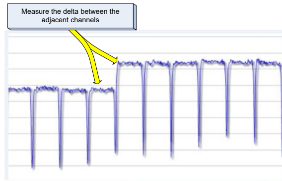
Figure 20 - Adjacent Misalignment in SC-QAM Channels in a CPE
