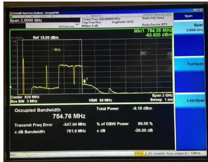
Figure 109 - Spectrum Analyzer Display of Downstream Signal with Low Laser Distortion, OFDM RxMER = 37 dB
