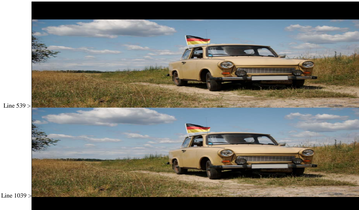
Figure 9 - TaB formatting with incorrect letterbox alignment
