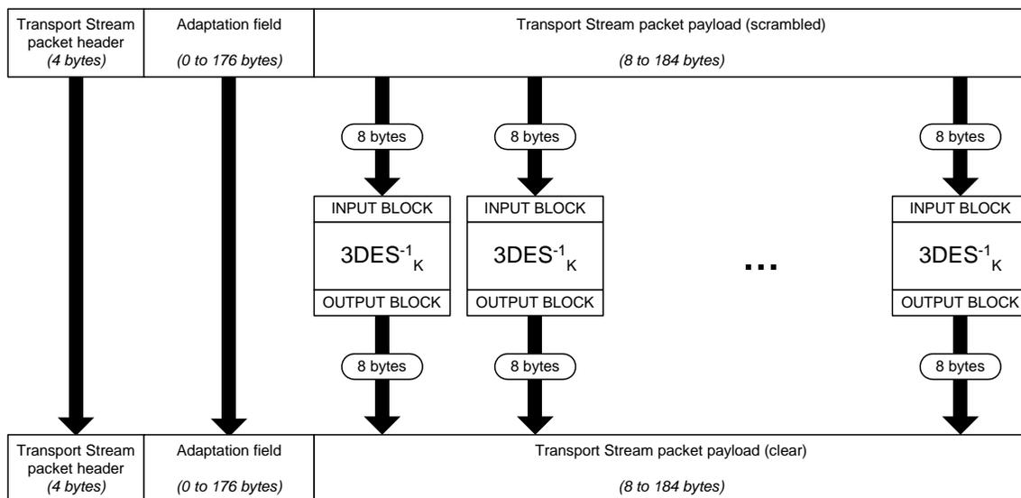
Figure B.3-5 - MPEG Transport Packet Descrambling, Case 1
