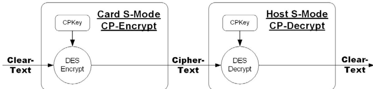
Figure 7-2 - S-Mode Encryption
