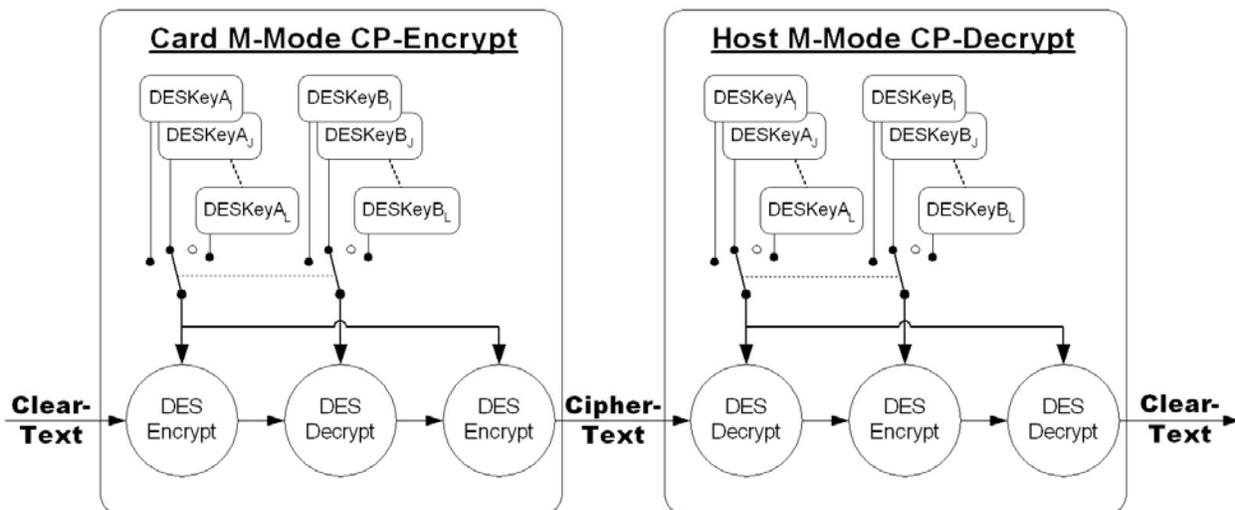
Figure 7-3 - M-Mode Encryption
