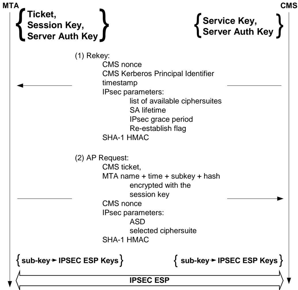
**Figure 9. Rekey Message to Establish a Security Parameter**
