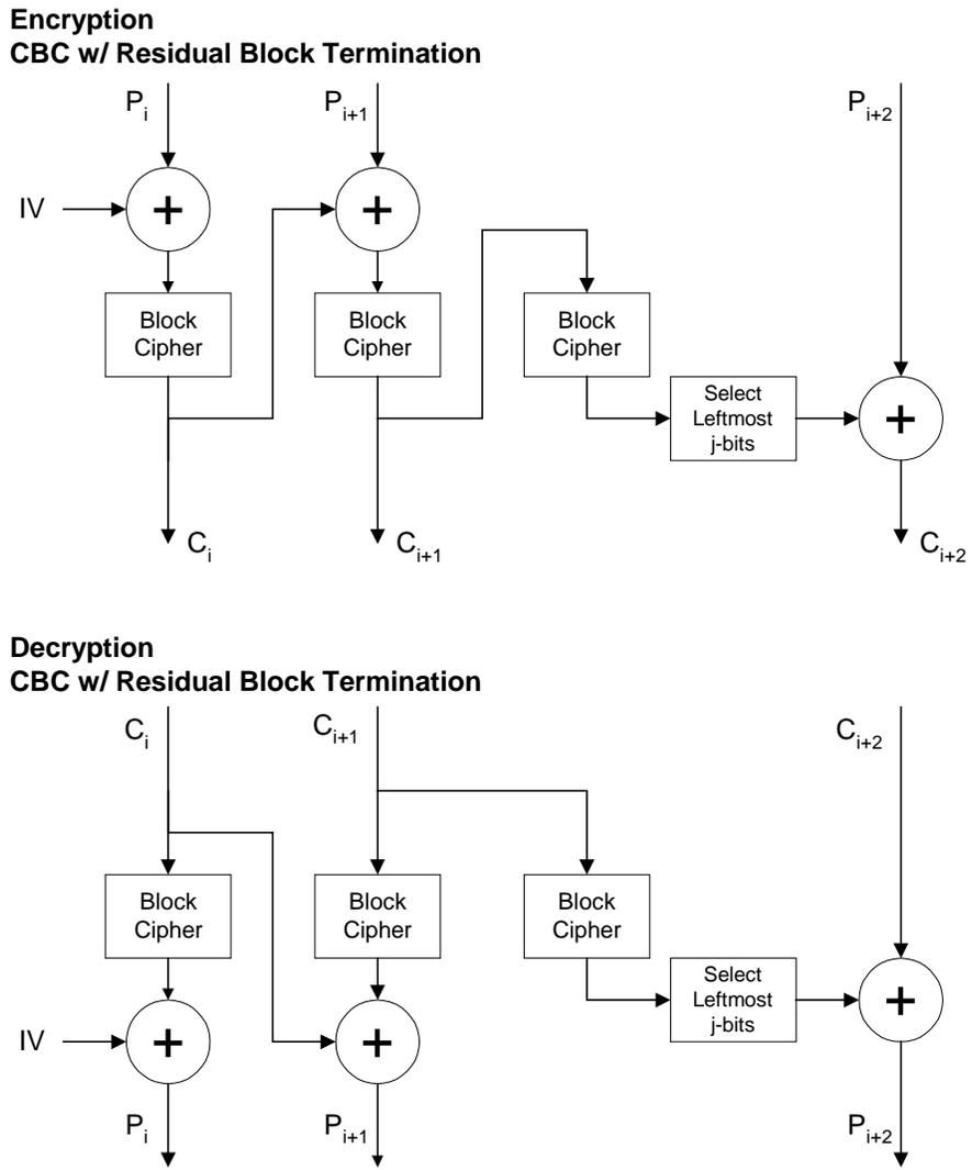
**Figure 28. CBC with Residual Block Termination**
