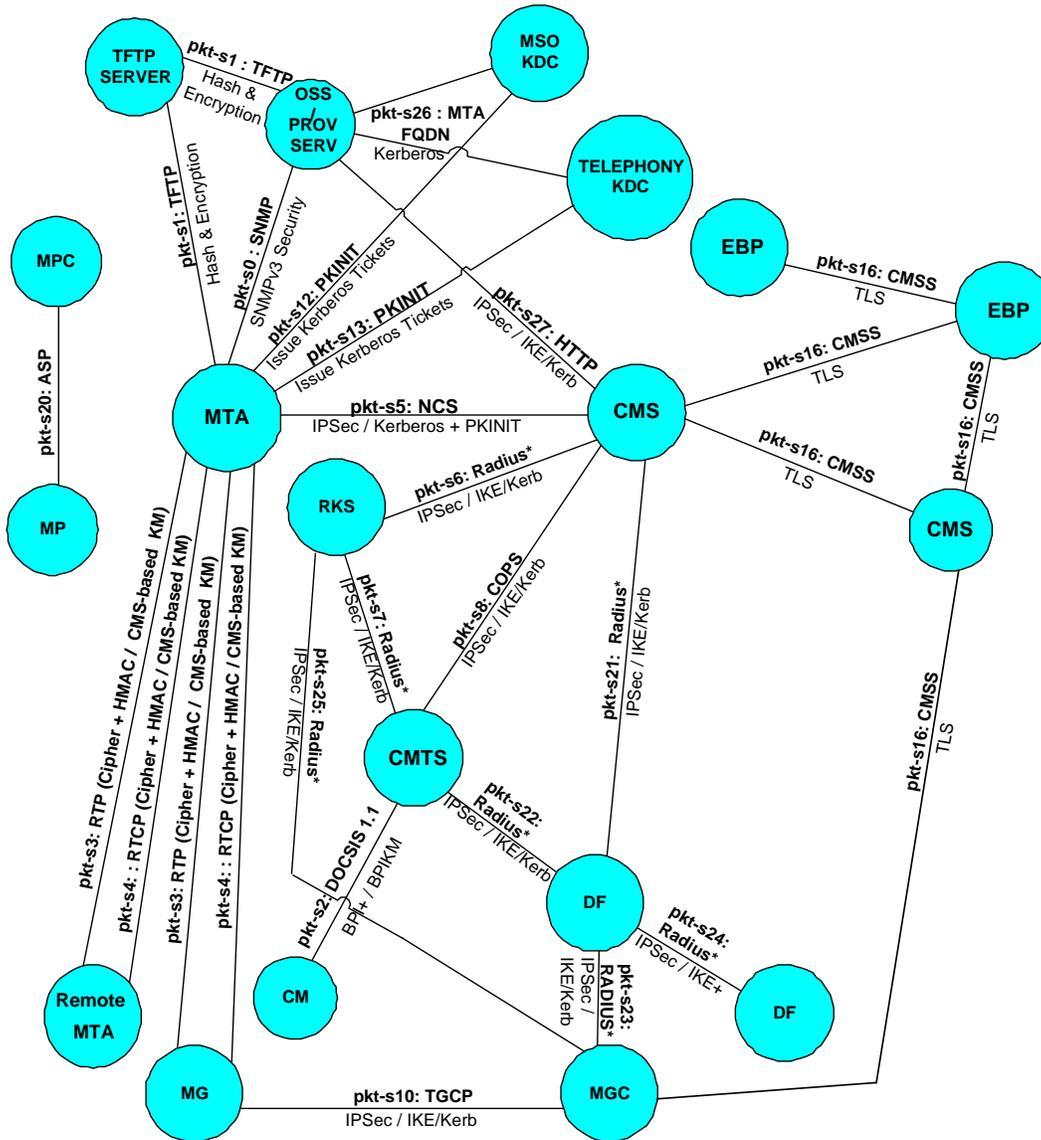
Figure 3. PacketCable Security Interfaces with Key-Management
