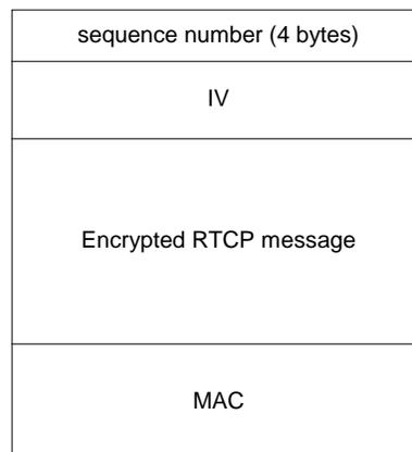
**Figure 19. RTCP Encrypted Packet Format**
