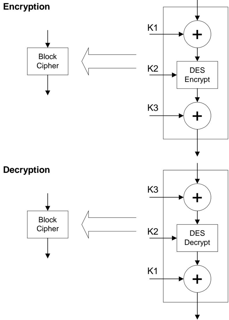
Figure 26. DESX-XEX as Block Cipher
