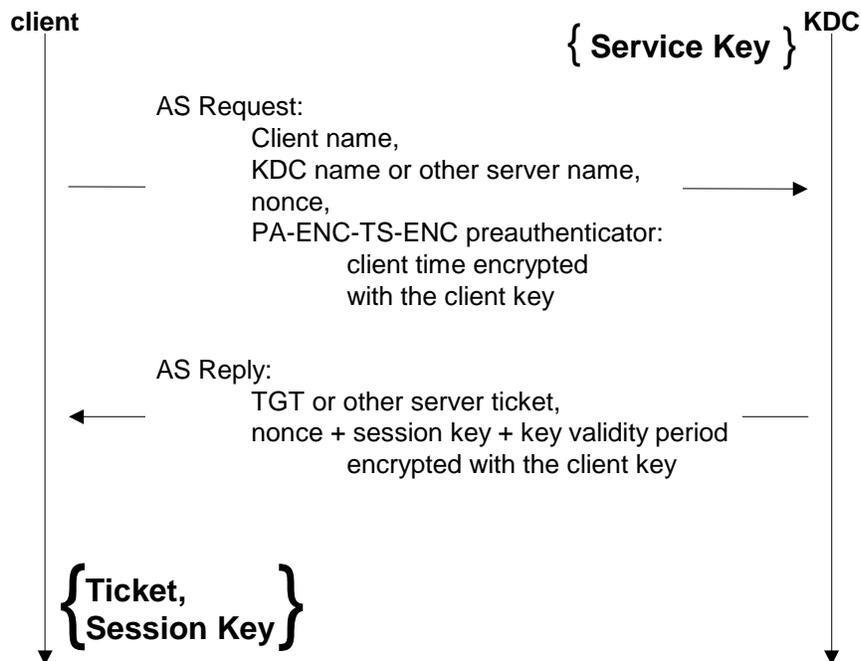
Figure 6. Symmetric-Key AS Request / AS Reply Exchange
