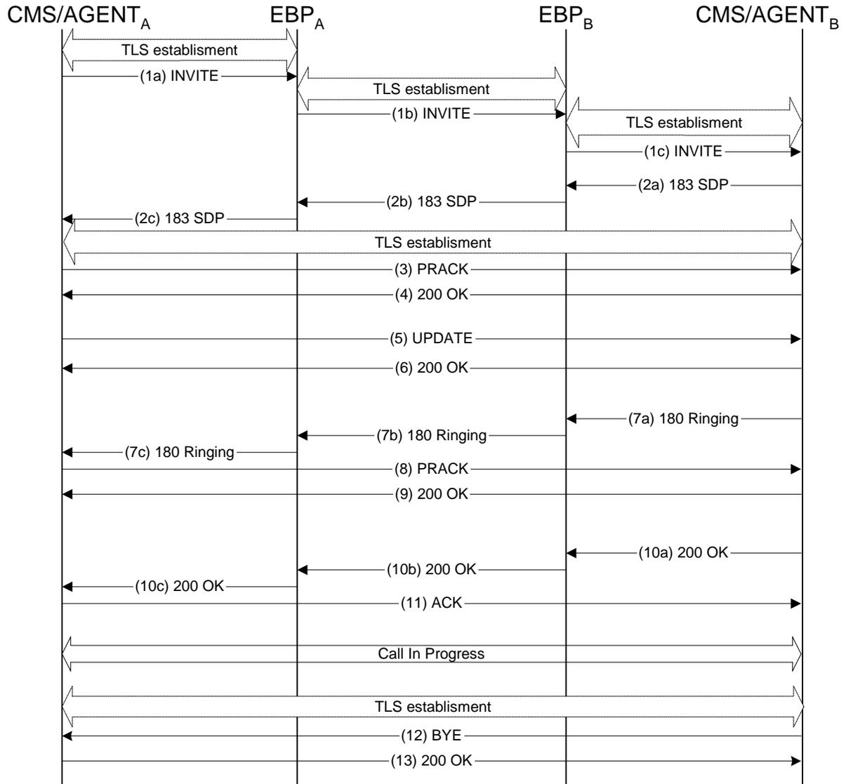
Figure 14. CMS – CMS Signaling Flow with Security
