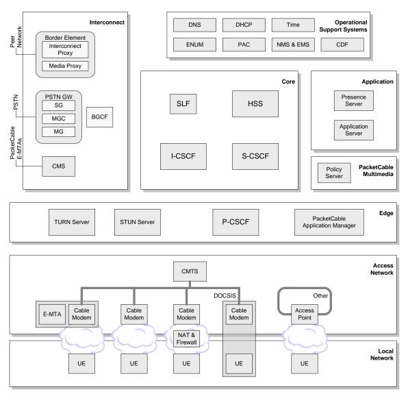
Figure 1 - PacketCable Reference Architecture
