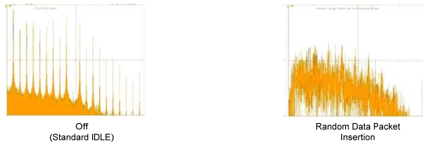
Figure 4 - Interference Spectra Without and With Raman Mitigation
