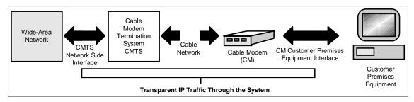
Figure 1–1 - Transparent IP Traffic through the Data-Over-Cable System
