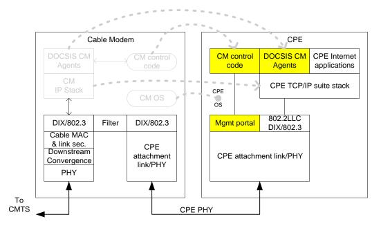
Figure C–1 - CPE Controlled Cable Modem (CCCM) functional migration
