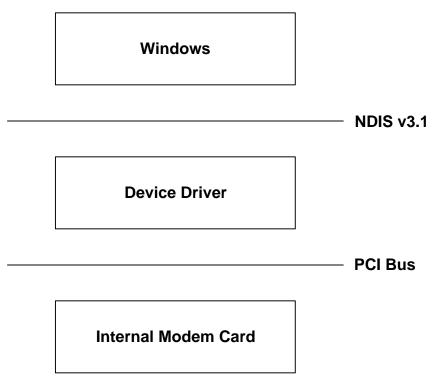
Figure 3–6 - PC Block Diagram
