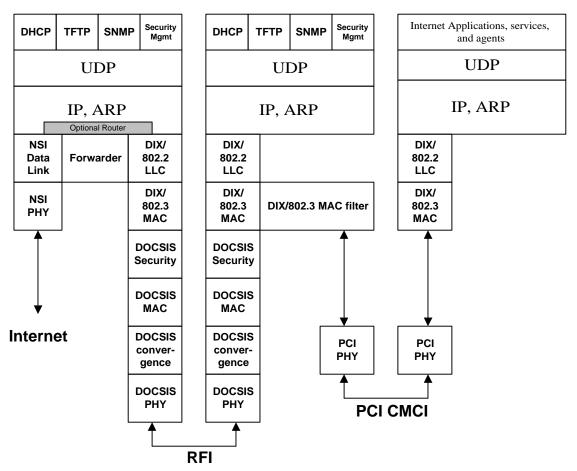
Figure 3–5 - End-to-End PCI Cable Modem Protocol Stack
