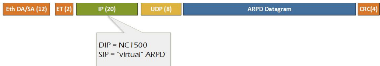
Figure 14 - CCAP Core to Network Controller Packet Format
