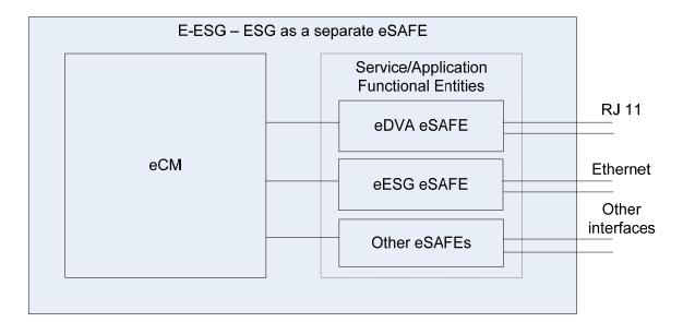
Figure 11 - Embedded ESG as a Separate eSAFE
