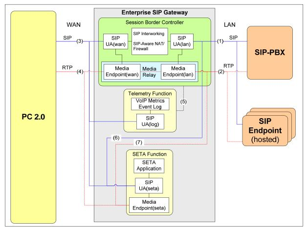
Figure 2 - ESG Block Diagram
