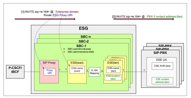
Figure 18 - SBC SIP Proxy Linked to a Single ESE(wan) Object
