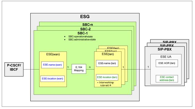
Figure 16 - Support for Multiple ESEs with Single ESE(wan)
