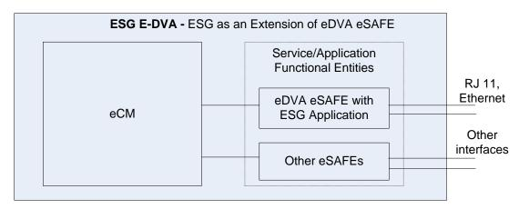
Figure 10 - Embedded ESG as an extension of eDVA eSAFE
