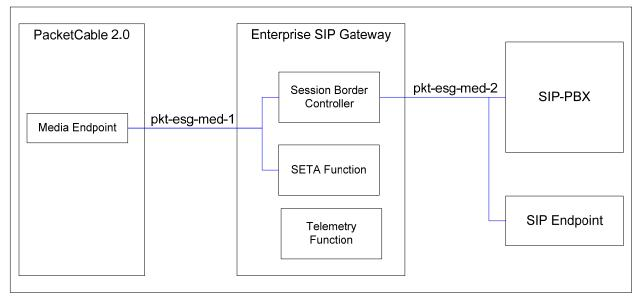
Figure 5 - ESG Media Reference Architecture
