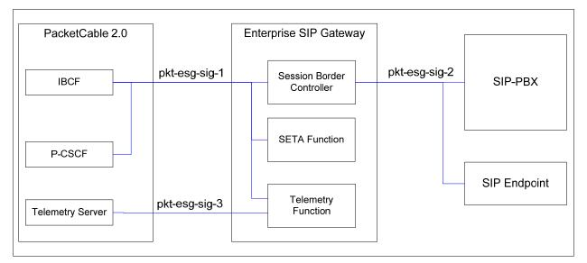
Figure 4 - ESG Signaling Reference Architecture
