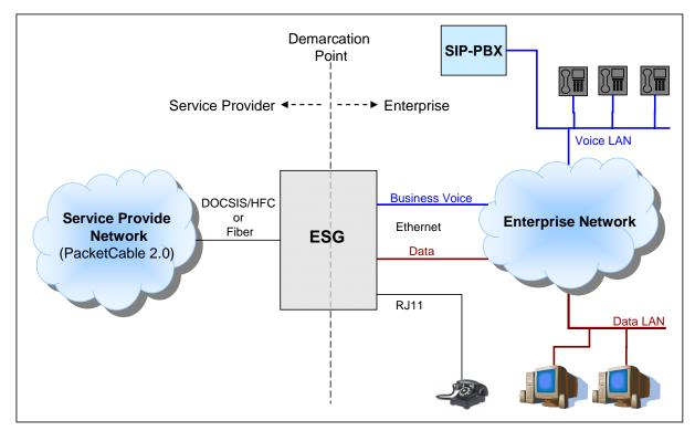
Figure 1 - ESG Network Architecture Overview
