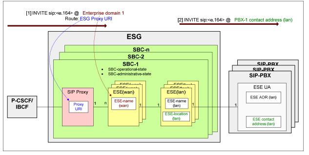
Figure 17 - SBC SIP Proxy Linked to Multiple ESE(wan) Objects
