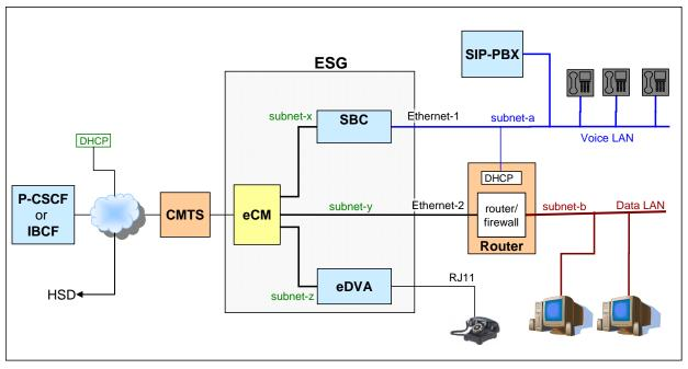
Figure 3 - ESG Deployment Option - Voice & Data on Separate LANs
