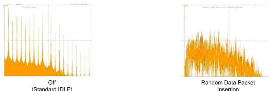
Figure 4 - Interference Spectra Without and With Raman Mitigation
